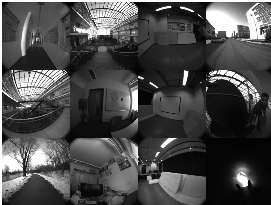
Figure 7.1: The TUM VI benchmark includes synchronized measurements from an IMU and a stereo camera in several challenging indoor and outdoor sequences. The cameras are equipped with large field-of-view lenses ( 195^\circ ) and provide high dynamic range images (16 bit) at high resolution (1 MP) with linear response function. The figure shows example frames from the dataset.
