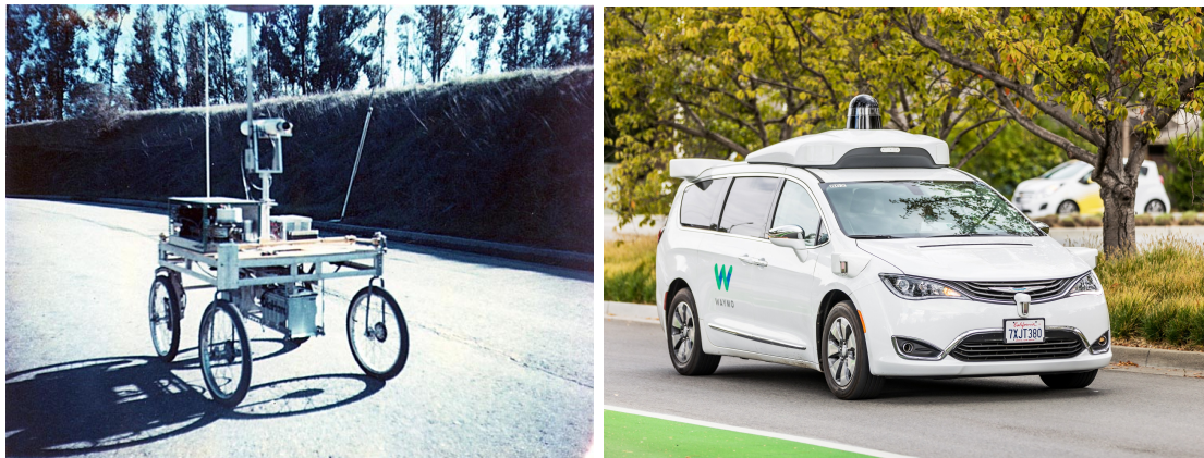
Figure 1.5: The Stanford AI cart from the 1970s shown on the left was one of the first robots to use cameras for navigation [90]. One of Waymo’s modern self-driving cars that have autonomously driven 3.5 million miles and have a 360-degree camera system among other sensors [129] is shown on the right. Illustrations taken from [90, 129].
