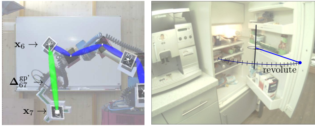
(a) online adaptation of the body schema (b) learned kinematic model of a fridge door
