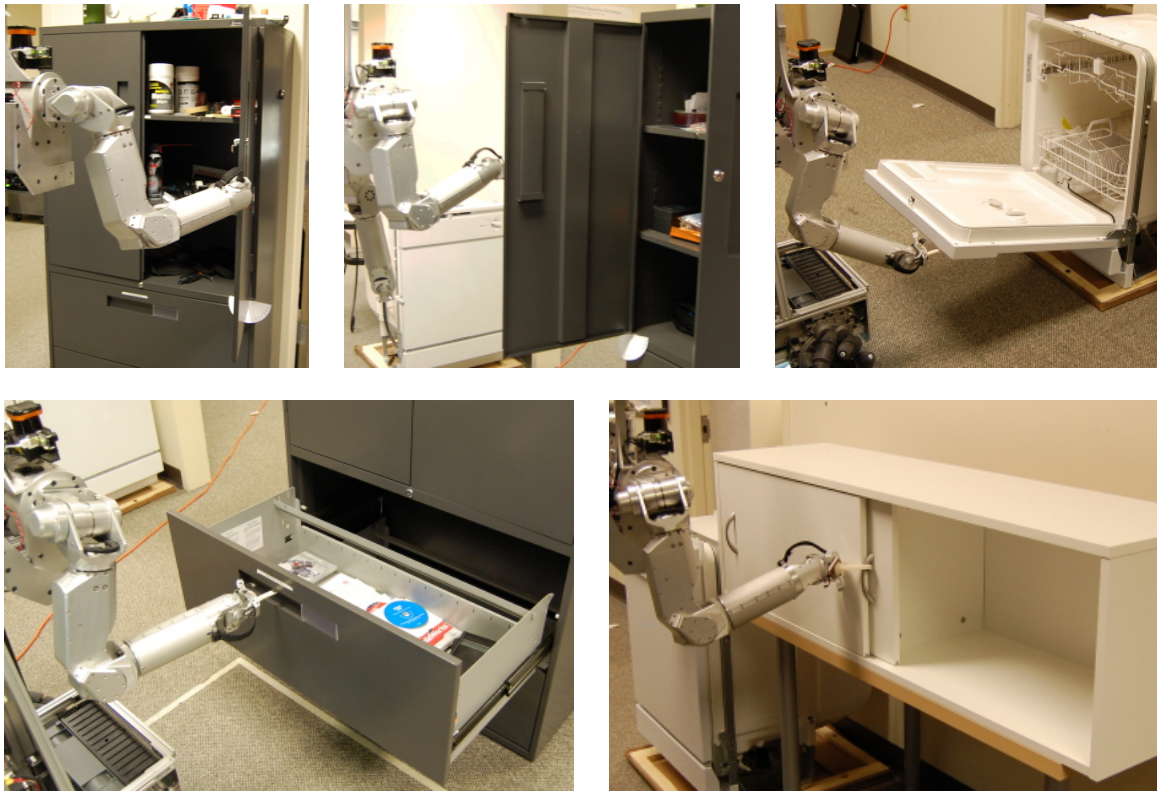
Figure 4.12: Images showing Cody at Georgia Tech operating the five different objects using the approach described in Section 4.3. Images courtesy of Jain and Kemp.
