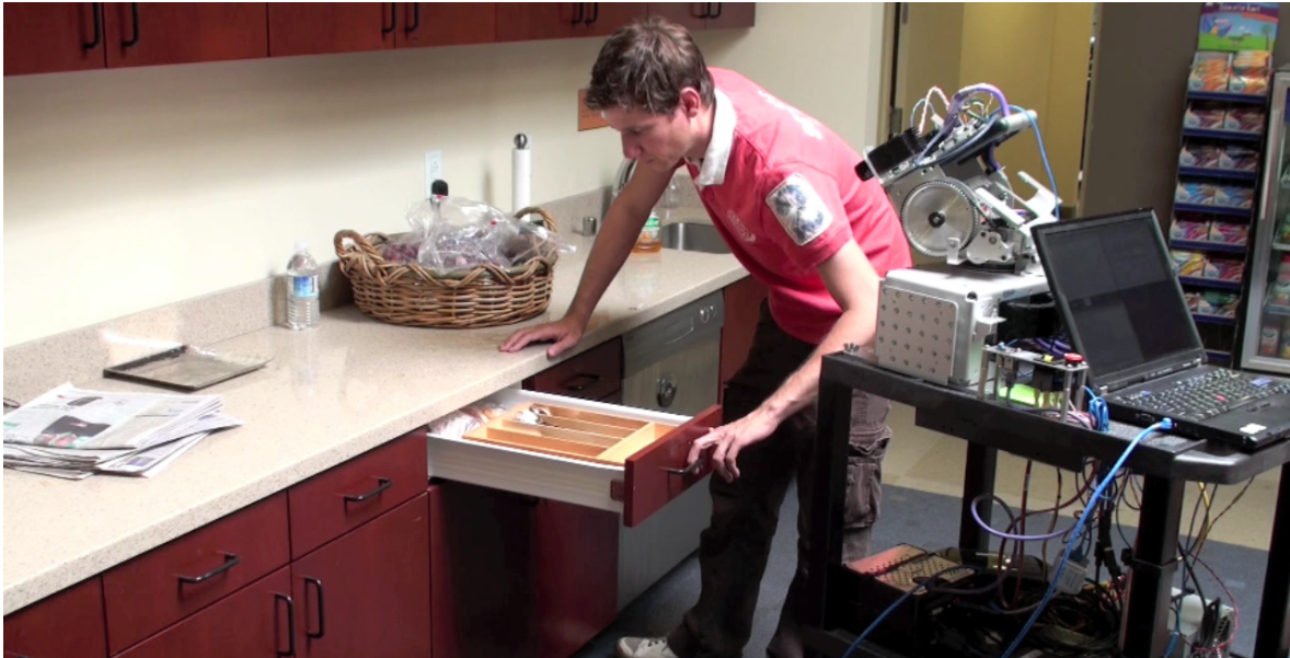
Figure 5.1: Experimental setup: the robot tracks the pose of a drawer in a sequence of dense depth images and infers its kinematic model.
