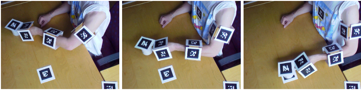
Figure 8.3: Human demonstration of a pick-and-place task. The trajectory is recorded both in task and joint space.
