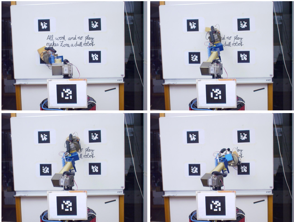
Figure 8.8: The reproduction of the board cleaning task by our robot. It imitates the zig-zag movement for cleaning the board with the sponge.
