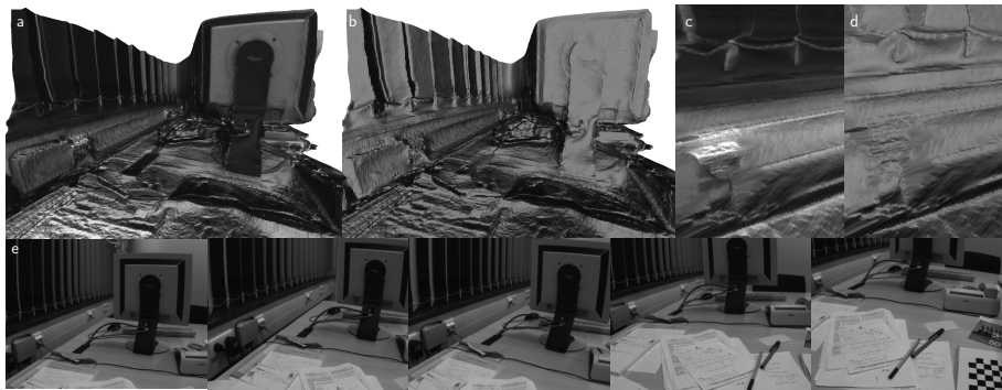
Fig. 2. Textured (a,c) and untextured geometry (b,d). Note the accurate reconstruction of small-scale details like the network socket and cords. (e) Images.
