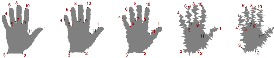
Fig. 6. Gaussian noise. The matching between an original hand and a hand added with Gaussian noise is visualized. From left to right the standard deviation is \sigma = 0, 0.5, 1, 3, 4 . At \sigma = 4 a matching starts to collapse (cf. point 4).
