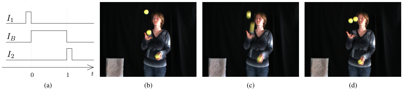
Fig. 1. Alternate exposure images: (a) exposure timing diagram of (b) a short-exposed image I_1 followed by (c) a long-exposed image I_B and (d) another short-exposed image I_2 .
