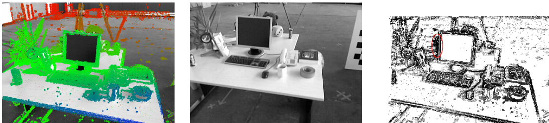
Figure 4.7: Left: semi-dense depth map of tracking reference image. Middle: new image to be tracked. Right: weight image in converged state in the reference image view; the brighter, the higher the weight is. The occlusion of the region left to the computer screen is visible as a black region (circled in red).
