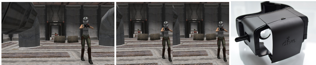
Figure 6.1: Left: screenshot of VR demo as displayed on a smartphone. Middle: screenshot of stereo mode, to be used with virtual reality goggles such as the Durovis Dive [12], shown on the right . The smartphone is inserted as display at the front of the goggles. 1
