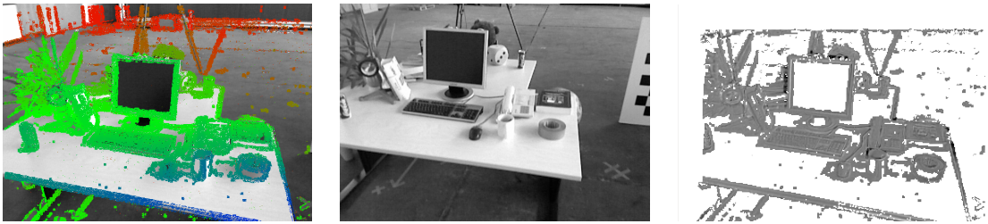
Figure 4.3: Left: semi-dense depth map of tracking reference image. Middle: new image to be tracked. Right: residual image in converged state in the reference image view; gray is the optimum. Occlusions are visible as darker or brighter spots, and the difference in field of view can be seen as there are no residuals for the upper and left parts of the image.
