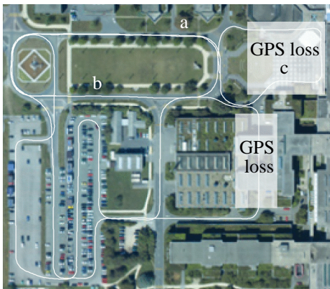
Fig. 5. Overlay of the estimated trajectory and the ortho-photo of the EPFL campus. The zones where the GPS was not available are highlighted. The total traveled distance is around 2300m. The labels (a), (b), and (c) identify areas which are later on referred to by Figure 6 and 7.
