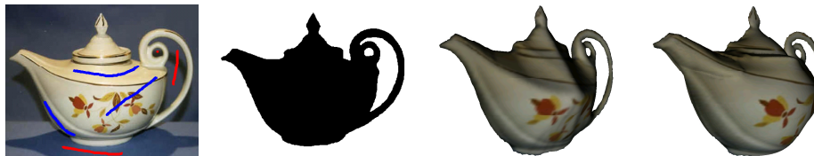
Fig. 2. Workflow of the proposed method: Input image with user provided seeds (foreground: blue, background: red), segmentation, reconstruction with default parameter settings, reconstruction with user-adapted parameter settings.
