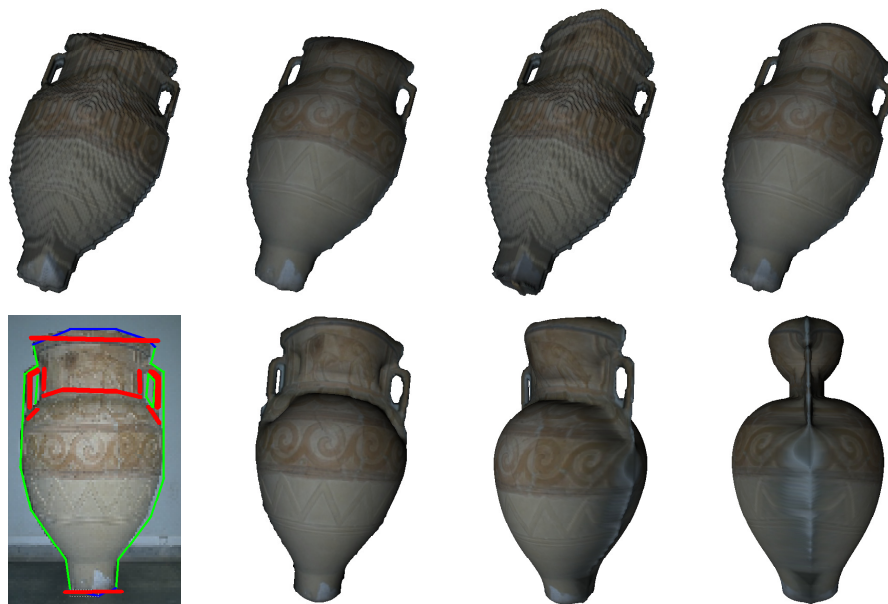
Fig. 4. Top row: height maps and corresponding reconstructions with and without marked sharp contour edges. Bottom row: input image with marked contour edges (blue) and line strokes (red) for local discontinuities which are shown right.
