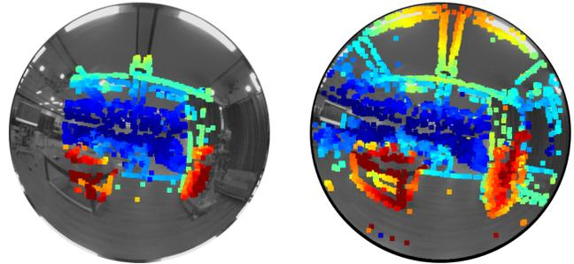
Fig. 1. **Top:** Active pixels in DSO for different camera models (left: pinhole, right: omnidirectional). With the pinhole model, DSO can only use a small part of the original fisheye image. In contrast, with the omnidirectional model, DSO can use pixels across the whole fisheye image. **Bottom:** Example of reconstructed map
