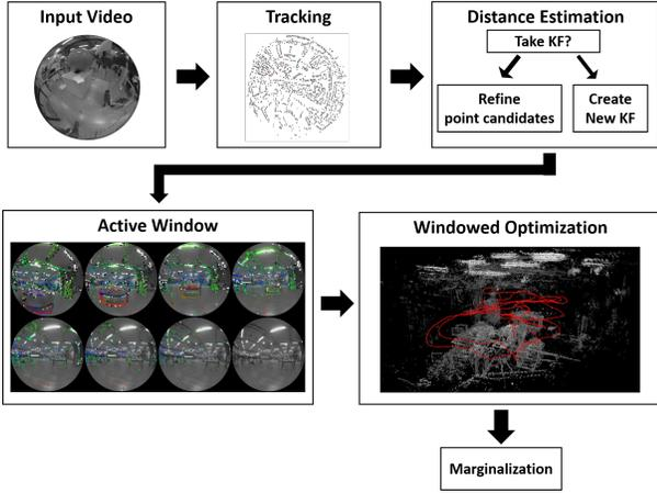
Fig. 4. System overview of omnidirectional DSO (OmniDSO).
