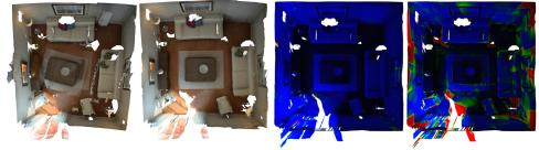
a) Without and with on-the-fly surface correction b) Surface completeness (5 vs. 60 frames per keyframe)
