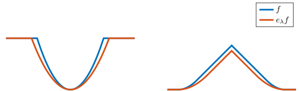
Figure 1: Illustration of nonconvex, nonsmooth Moreau envelopes e_\lambda f (red curves). The two depicted piecewise quadratic loss functions f (blue curves), are invariant under Moreau-Yosida regularization up to rescaling. Left: The Moreau envelope of a truncated quadratic loss, given as f = \min \{\nu, (\cdot)^2\} for \nu > 0 , is a nonsmooth, nonconvex truncated quadratic loss with rescaled slope. Right: The Moreau envelope of a symmetric Huberized hinge loss is a nonsmooth, nonconvex symmetric Huberized hinge loss with rescaled slopes of the quadratic pieces given as e_\lambda f = \min_{\theta \in \{-1, 1\}} e_\lambda(1 - (\cdot)\theta)_+ .
