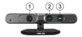
Figure 2.3.: ASUS Xtion PRO LIVE camera: ① IR projector ② RGB camera ③ IR camera [26]
