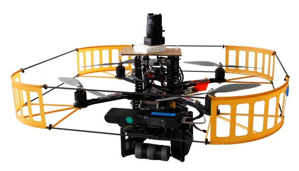
Figure 2.2.: AscTec Pelican quadrocopter with payload: the Autopilot Board, the Mastermind Board, a monocular grayscale camera and an ASUS Xtion PRO LIVE RGB-D camera.
