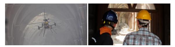
Figure 1.1.: Quadrocopter with RGB-D camera inspecting a church damaged during an earthquake (left). The quadrocopter is entirely controlled by human operators (right). [2].
