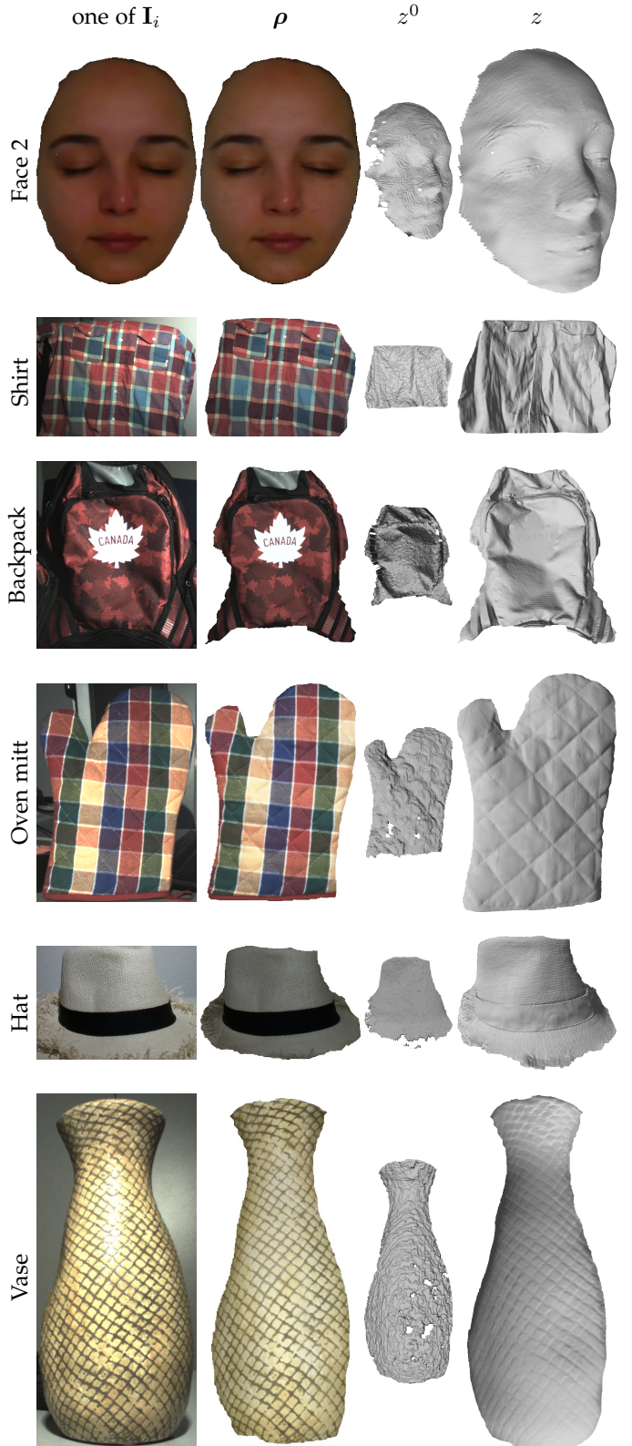
Fig. 6: Qualitative results of our uncalibrated photometric stereo-based method, on real-world data captured using a RealSense D415 (“Hat” and “Face 2”) or an Xtion Pro Live (five other datasets).
