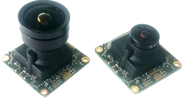
Figure 2. Cameras used to capture the dataset. Left: narrow lens ( 98^\circ \times 79^\circ non-rectified field of view), right: wide lens ( 148^\circ \times 122^\circ non-rectified field of view).
