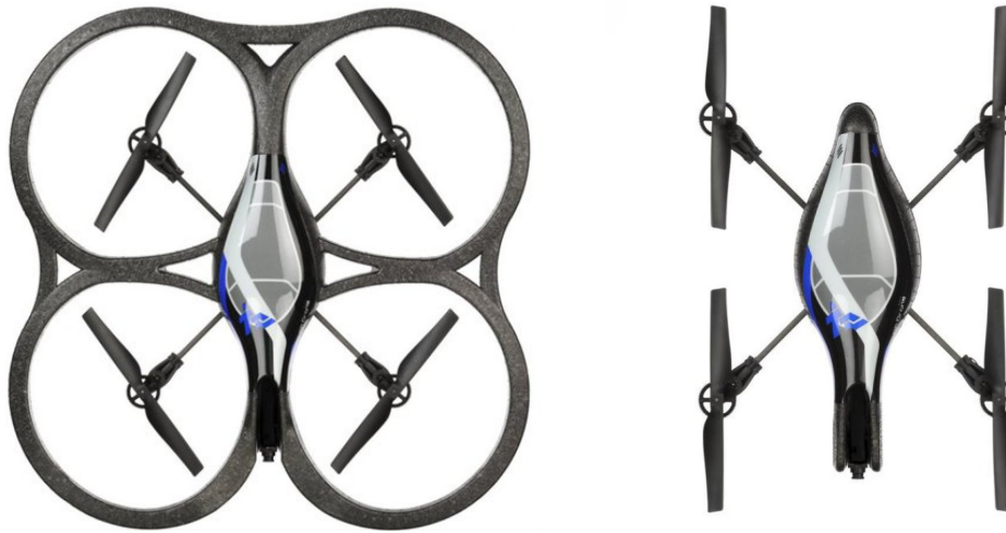
Figure 2.2. The Parrot AR.Drone with indoor-hull (left) and outdoor-hull (right).
