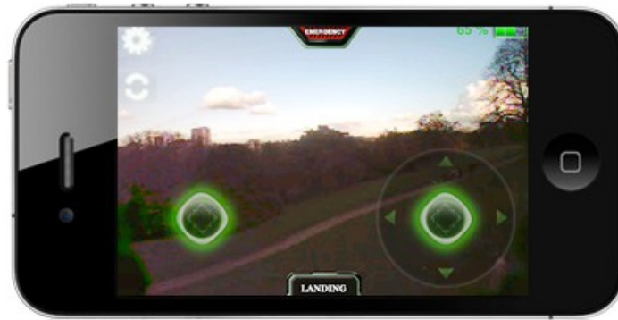
Figure 2.4. The AR.FreeFlight App running on an iPhone. While for horizontal movement the device is simply tilted in the respective direction, altitude and yaw rotation are controlled using the button on the right side.
