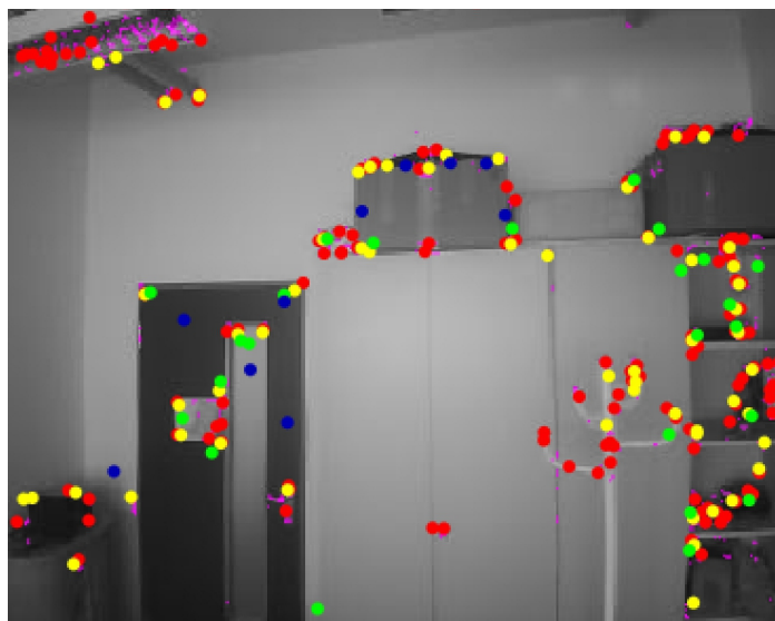
Figure 3.3. Locations of keypoints used by PTAM for tracking. The color represents the pyramid-level on which the keypoints was found: blue dots correspond to coarse and large patches, while red dots correspond to very fine and small keypoints.
