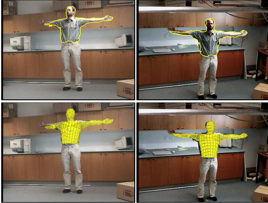
Fig. 11.4. Result with a global Parzen estimator instead of the suggested local region statistics. The same initialization as in Figure 11.2 was used. Top row: Estimated contour. Bottom row: Estimated pose. Local differences between foreground and background are not modeled. With the global model, the right arm of the person better fits to the background.
