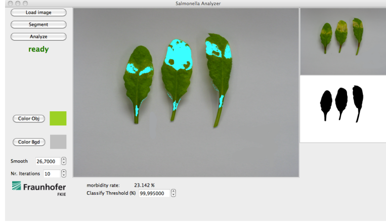
Figure 3: Screenshot of the algorithm GUI. In the center the marked pixels are displayed. On the right the input image and the segmentation result can be seen. On the left and at the bottom control parameters can be set.
